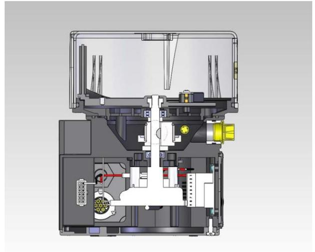
*The gear motor is protected by means of an IP-56 protection degree covering (NYLON PA6 +30% FIBERGLASS). The seal is guaranteed from well-mounted "o"-ring.*
